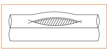
Fig: 2.2.6 Ductile Burst is Preceded by Outward Bulging
