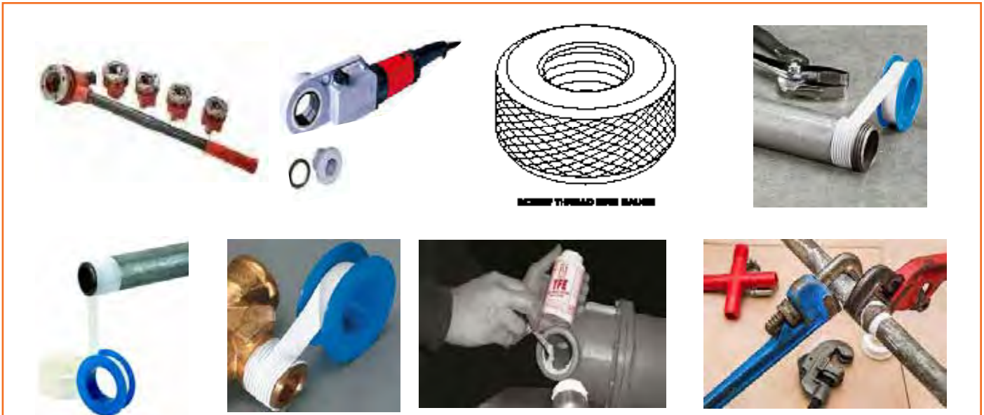
Fig. 1.7.31 GI – piping threading and assembling
