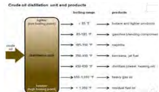
2.2.2 illustration of crude oil products and their boiling range.
