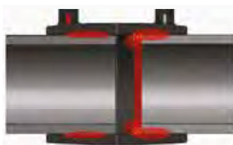
Fig. 2.4.18 Short stab – Incorrect assembly
