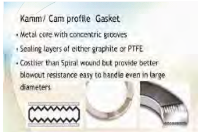
Fig. 1.5.70 Camprofile gasket
