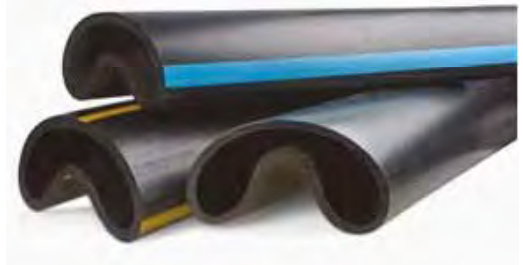
Fig. 2.4.3 Damaged Pipe ends
