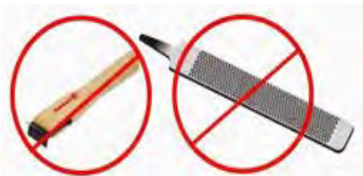
Fig. 2.4.10 Not Recommended hand tools for PE
