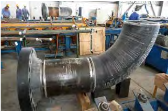
Fig. 1.7.36 Pipe to Elbow Fitup and Alignment
