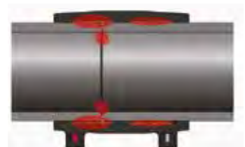
Fig. 2.4.19 Mis-stab – Incorrect assembly
