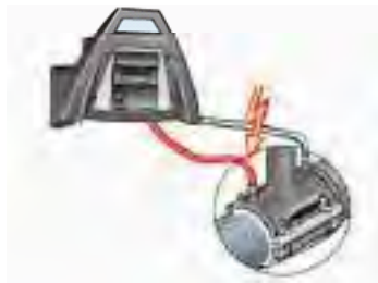
Fig. 2.6.66 Connecting terminal cable
