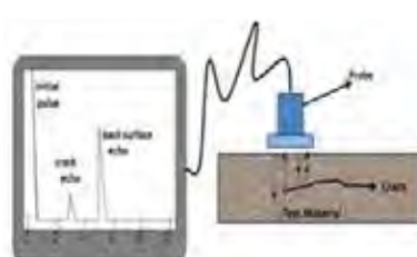
Fig. 1.8.94 Typical UT testing set up and screen pattern
