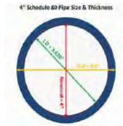
Fig. 1.2.23 – Pipe - OD & ID indication
