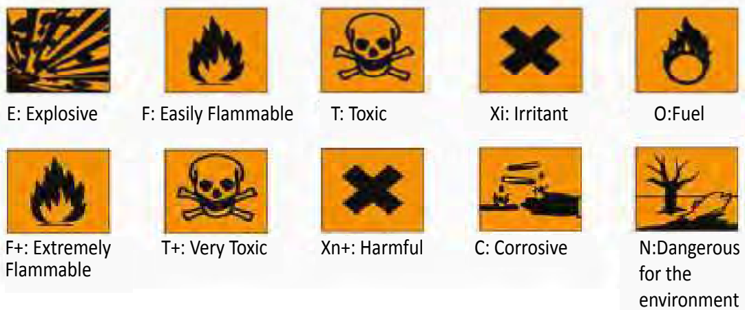
Fig. 4.1.37 Different hazard signage
