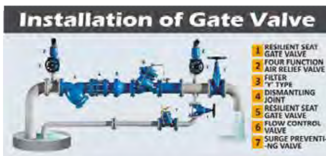
Fig. 1.5.79 Typical Gate Valve installation arrangement
