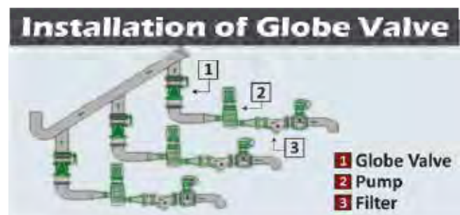
Fig. 1.5.80 Typical Globe Valve installation arrangement
