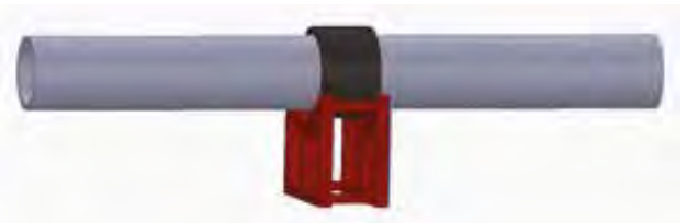
Fig. 2.6.41 Incorrect support placement
