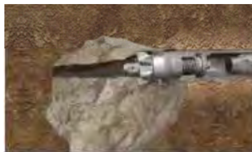
Fig. 2.1.19 Impact moling in rock / hard surface
