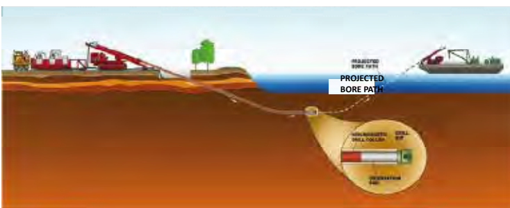
Fig. 2.1.22 Shore approach pilot hole drilling
