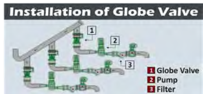
Fig. 1.5.80 Typical Globe Valve installation arrangement
