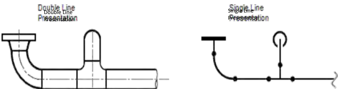
Fig. 1.2.19 Example of a single line and double line representation of a piping
