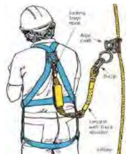
Fig. 4.1.39 Working at heights
