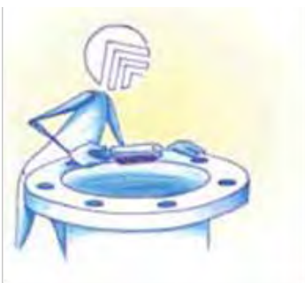
Fig. 1.7.48 Checking flange faces
