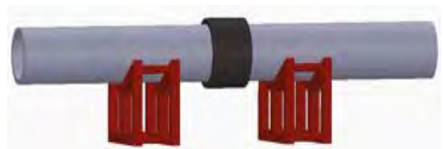
Fig. 2.6.40 Correct support placement
