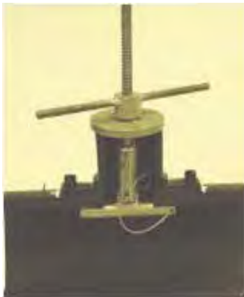
Fig. 2.6.86 Tightening T clamp
