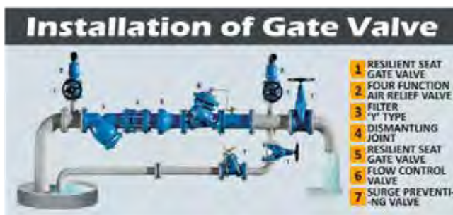
Fig. 1.5.79 Typical Gate Valve installation arrangement
