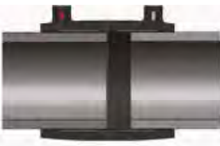
Fig. 2.4.18 Short stab – Incorrect assembly
