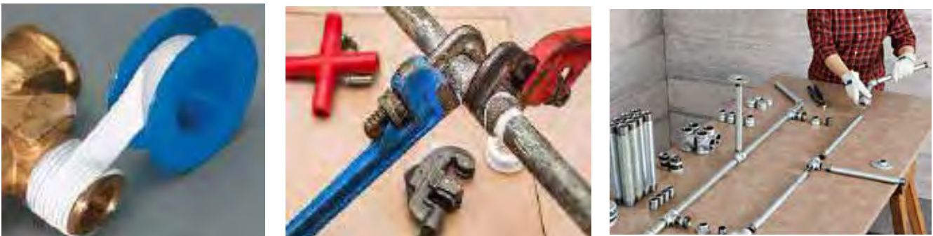
Fig. 1.7.30 Threaded Pipe Joint assembly
