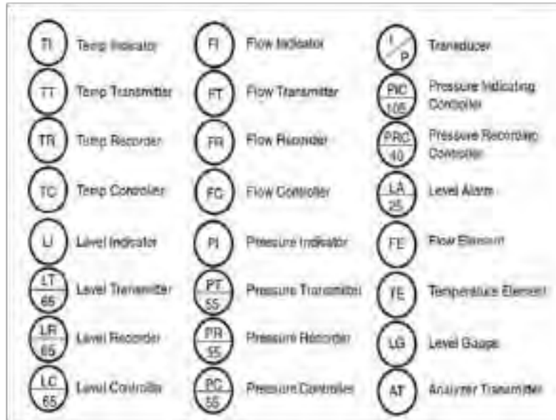
Fig. 1.2.36 Piping Instrument Symbols for Isometrics
