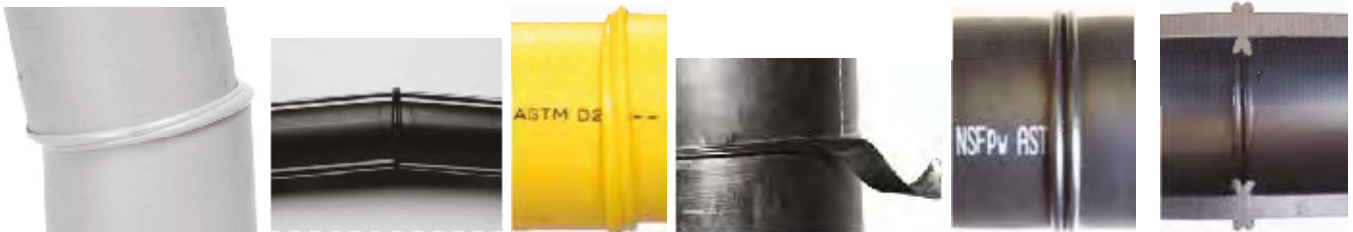
Fig. 2.5.21 Unacceptable mis alignment
