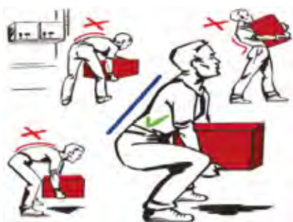
Fig. 4.3.13 Unsafe act of lifting too big
