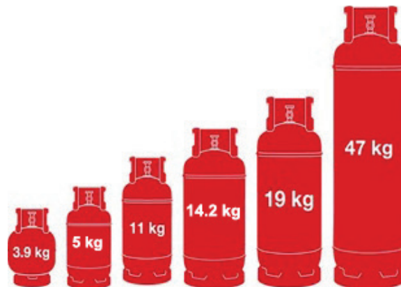
Fig. 2.1.7. LPG cylinders sizes and capacities
