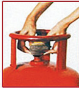
Fig. 2.5.14. Fit the pressure regulator on cylinder valve
