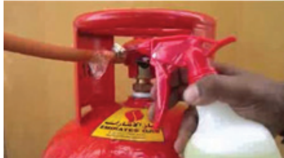
Fig. 2.5.7. Check LPG leakage with soap solution
