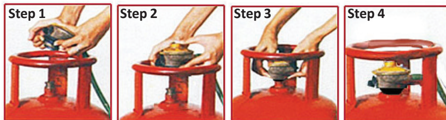
Fig. 2.3.9. Fit the pressure regulator on cylinder valve
