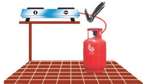
Fig. 2.5.4. Install cylinder in ventilated area
