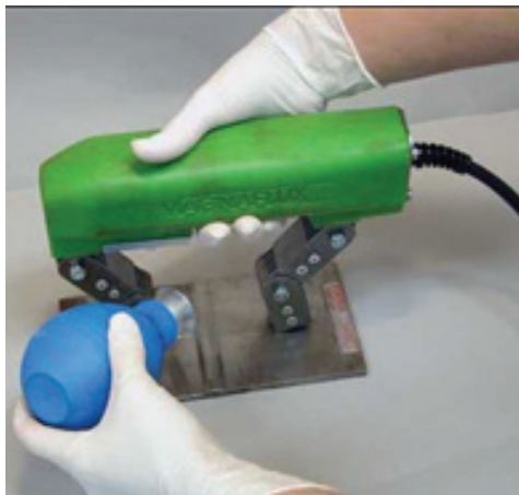
Figure 4.15.1_7 Magnetic particle testing
