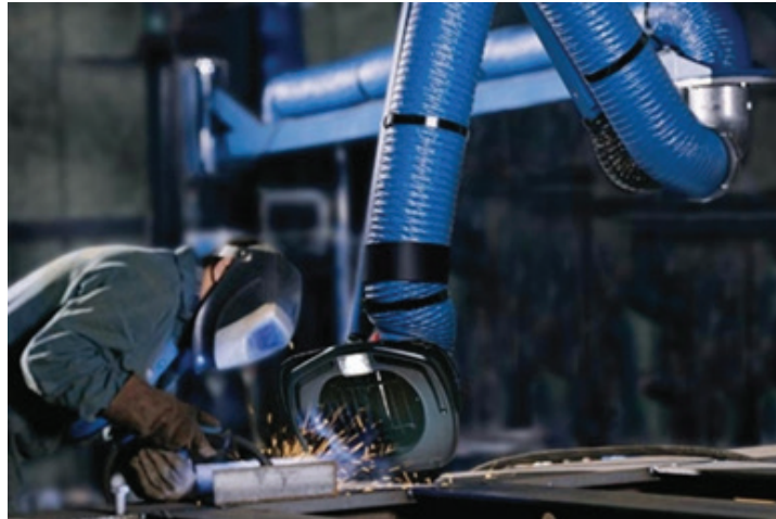
Figure 7.1: Local Exhaust Ventilation
