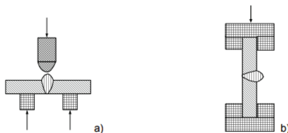
Figure 4.15.1_3 : Schematics of Free Bend test
