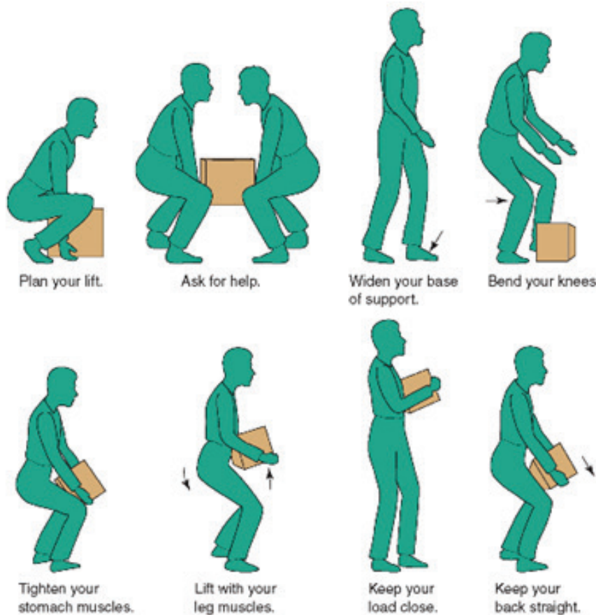
Figure 7.10: Safe lifting techniques
