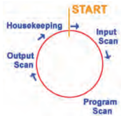
Figure 3.5_2: Operation system of PLC
