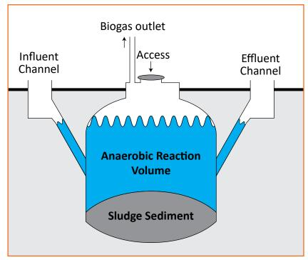
Fig: 2.1.1 Bio gas (diagram)
