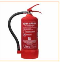
Instead of a jet nozzle a spray nozzle is used, with a higher pressure, which creates a fine spray. This allows for a given quantity of water to have a considerable increase in the surface area presented to the fire. This makes extinguishing more efficient by more rapid extraction of heat, formation of steam etc. They can also contain surfactants which help the water penetrate deep into the burning material which increases the effectiveness of the extinguisher.
