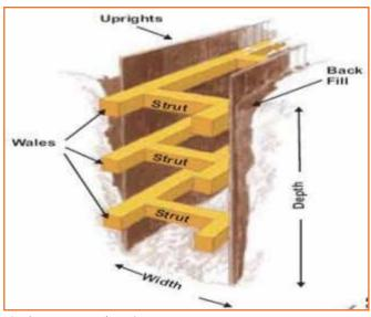
Fig: 2.1.17 Excavation Diagram
