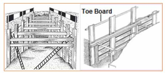
Fig: 2.1.16 Safety Precaution in Excavation
