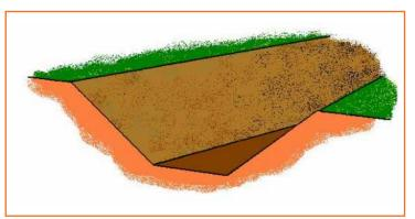
Fig: 2.1.9 Sloped Trench
