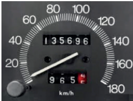
Trip Meter Records distance covered in a trip, can be reset by pressing of the knob. Some models are equipped with up to three different trip meters.
