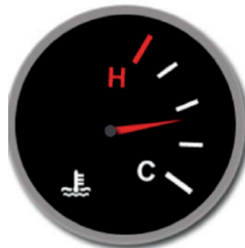
Temperature Gauge Indicates temperature of engine coolant. In case engine temperature goes up it is indicated by needle going towards H mark or temperature lamp lights up.
