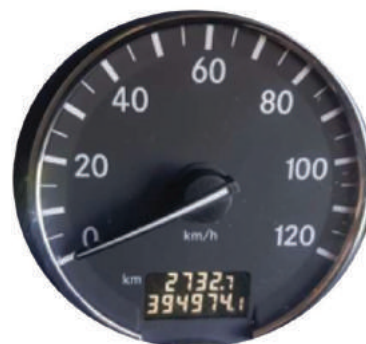
Odometer Records total distance covered by the vehicle.
