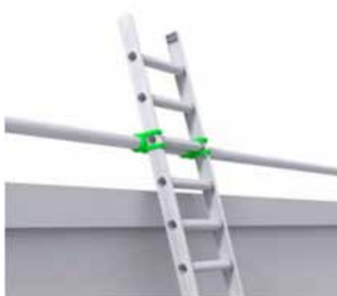
Figure 3.2.3: Tying the ladder above the stiles to work on and not gaining access
