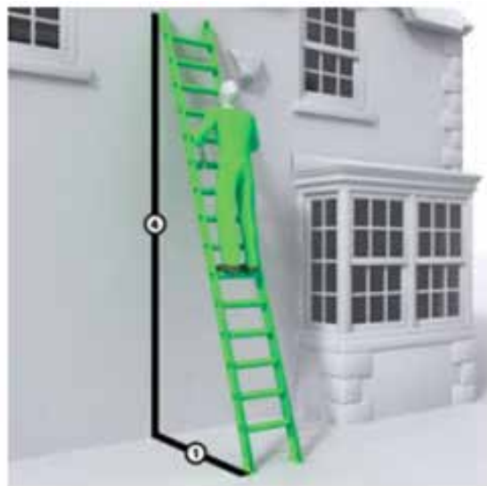
Figure 3.2.8: Right 1 in 4 angle shown with the help of a ladder
