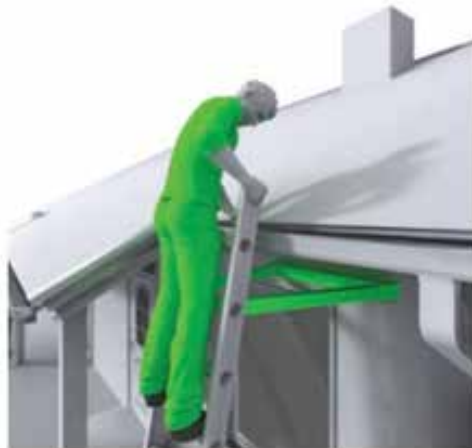
Figure 3.2.5: Taking the help of stand-off devices to get a strong resting point.
