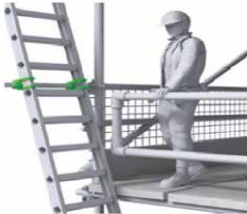
Figure 3.2.1: Tying the extension ladder and ensuring that it at least 3 feet higher than the supporting point
