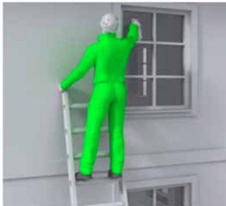
Figure 3.5.7: Following 3 point contact and not overreaching the work area
