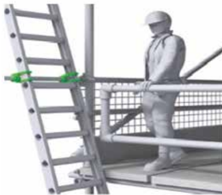
Figure 3.5.1: Tying the extension ladder and ensuring that it at least 3 feet higher than the supporting point
