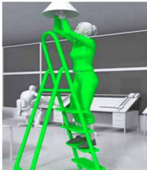
Figure 3.5.4: Ensuring that both the legs are on the same platform (step) with the knees supported to the stepladder and availability of handhold
