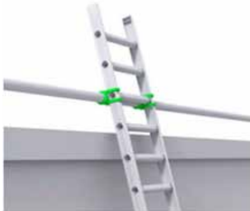
Figure 3.5.3: Tying the ladder above the stiles to work on and not gaining access
