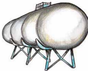
Figure 3.2.5: Second example of confined space
