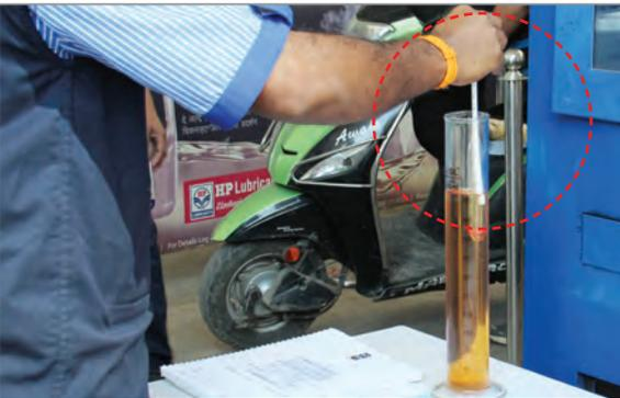
Fig. 2.1.20. Checking the density of a fuel
