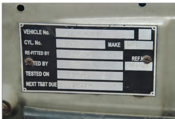
Fig. 3.2.1. CNG compliance plate
