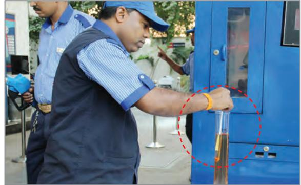
Fig. 2.1.19. Using calibrated hydrometer, thermometer
