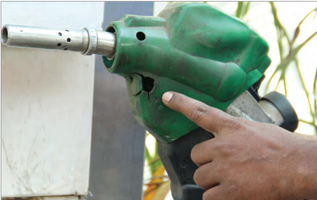
Fig. 3.2.2. Defective nozzle should be avoided
