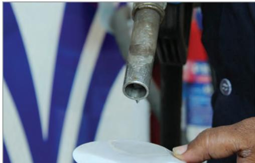
Fig. 2.1.14. Dispense a drop of petrol on the filter paper from the nozzle
