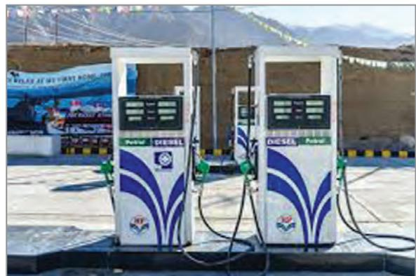
Fig. 2.2.1. Dual pump dispensing unit
