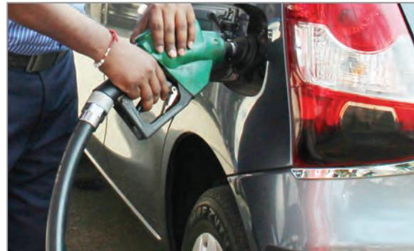
Fig. 2.3.2. Hose at a safe distance from the vehicle
