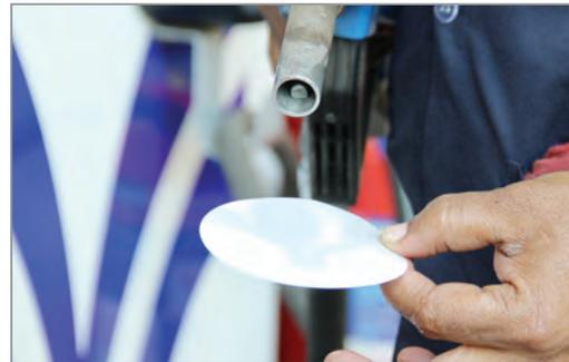
Fig. 2.1.15. Petrol evaporating from filter paper
