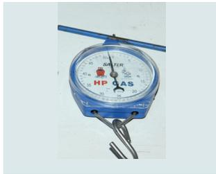
Fig. 2.2.12. Portable weighing machine
