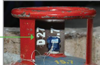
Fig. 3.2.8. Due date for testing
