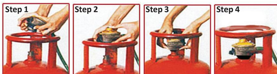
Fig. 2.3.14. Fit the pressure regulator on cylinder valve
