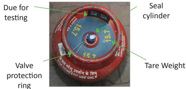
Fig. 3.1.2. Cylinder inspection
