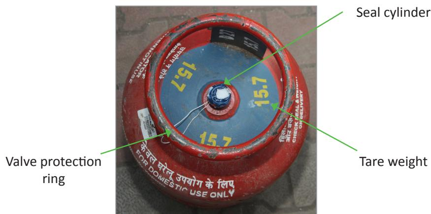
Fig. 2.2.2. Cylinder inspection
