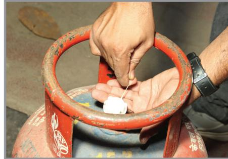
Fig 2.3.5 Open the safety cap
