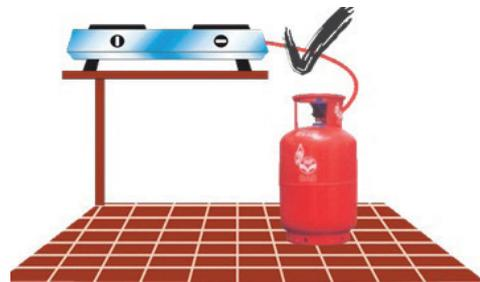
Fig. 3.1.4. Install cylinder in ventilated area
