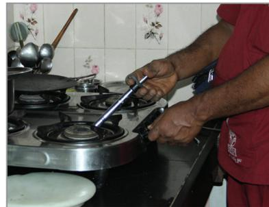
Fig 2.3.10 Check the cylinder connection
