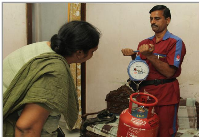
Fig 2.3.3 Show the weight of the filled cylinder
