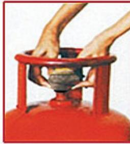
Fig. 3.2.12. Fit the pressure regulator on cylinder valve
